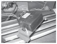
**25)** Connect the ground wire to the DC Sparker mounting bracket.
